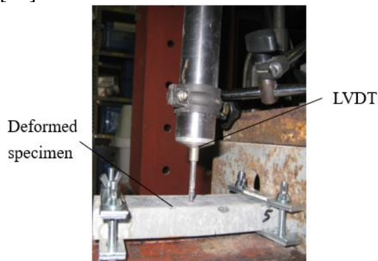
Figure 4 Measuring deflection using LVDT
